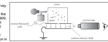
droplets become charged. The droplets fall through the chamber into the area between the metal plates. The voltage is turned off initially, and all droplets fall due to gravity. Once the voltage is turned on, the electrical force on charged droplets counteracts the gravitational force, and some drops begin to rise. A single droplet is selected by alternately turning on and off the voltage. The uncharged droplets fall to the bottom.
